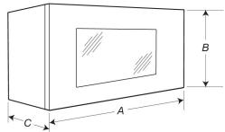
A. 29<sup>7</sup>/<sub>8</sub>" (76.1 cm) B. 17<sup>7</sup>/<sub>8</sub>" (45.4 cm) C. 12<sup>1</sup>/<sub>8</sub>" (31.3 cm)
