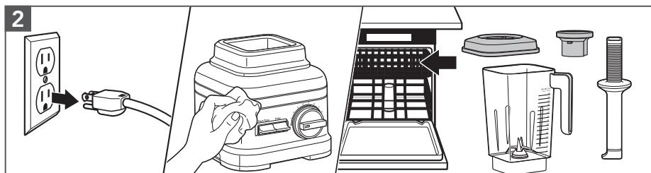
Unplug the Blender before cleaning. Wipe the Base and the cord with a warm, damp cloth and dry with a soft cloth.
