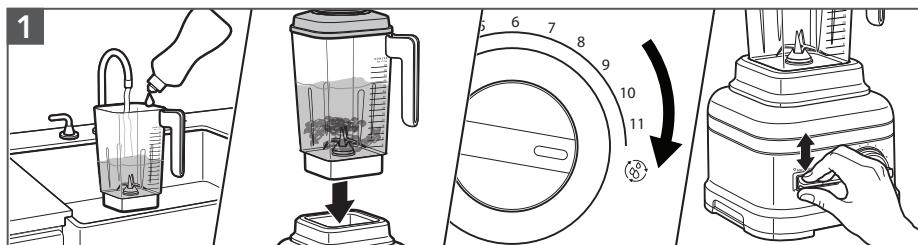
Unplug the Blender. Empty the Blender Jar. Fill half of the jar with water and add 3-4 drops of liquid dish-washing detergent. Place the Blender Jar with Lid on the Blender Base.
