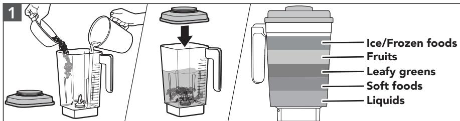
Put the items to blend into the Blender Jar. Secure the Lid with the Ingredient-measuring cap.
