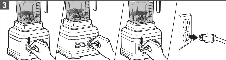
Flip the **Start/Stop** up or down to start. Turn the Control Dial to your desired speed. See the "Blender Function Guide" for more details. When finished, flip the **Start/Stop** up or down to stop. Unplug the Blender before removing Blender Jar.
