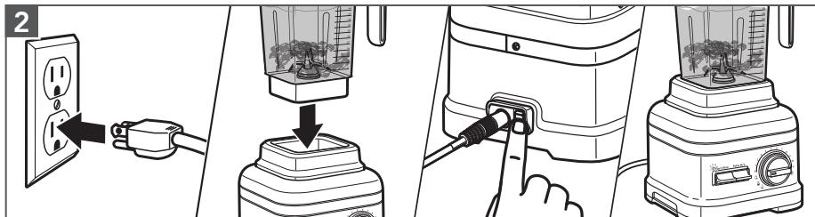
Plug the Blender into a grounded 3 prong outlet. Place the Blender jar on the Base. Flip the power switch to On (I). The Status Indicator Light will flash, indicating that the Blender is in Standby mode and ready.
