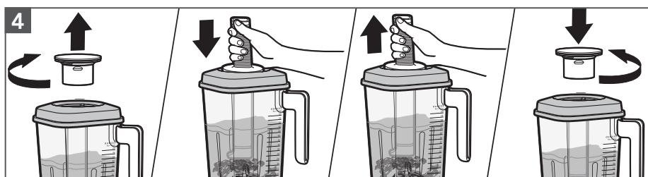
**Using the Tamper:** Remove the Ingredient-measuring Cap only. Stir or press contents down towards the Blade. When finished, replace the cap before resuming blending.
