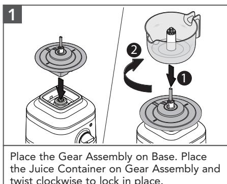
Place the Gear Assembly on Base. Place the Juice Container on Gear Assembly and twist clockwise to lock in place.
