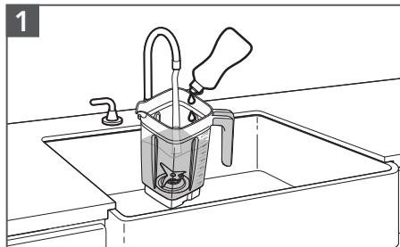
Fill half of the Jar with warm water and add 1 or 2 drops of dish-washing liquid. Place the Jar on the base. Secure the Lid and Lid Center Cap.
