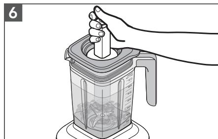
**Tamper accessory:** Remove the Lid Center Cap only. Stir or press contents down towards the blade. Then, place the Lid Center cap back before resuming blending.
