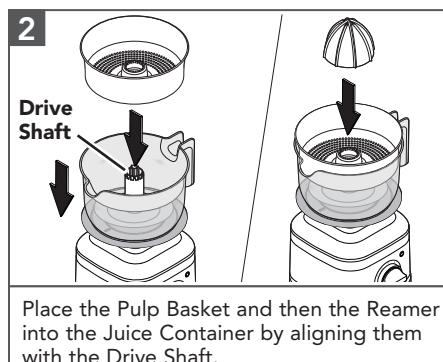
Place the Pulp Basket and then the Reamer into the Juice Container by aligning them with the Drive Shaft.
