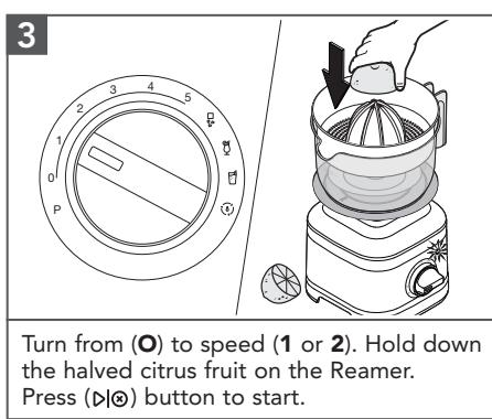
Turn from (O) to speed (1 or 2). Hold down the halved citrus fruit on the Reamer. Press (▷|∅) button to start.
