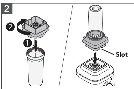
Secure the Blade Assembly on the Jar and rotate it clockwise until it is tight. Place it on the Base.
