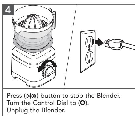
Press (▷|∅) button to stop the Blender. Turn the Control Dial to (O). Unplug the Blender.
