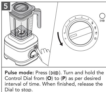
**Pulse mode:** Press (▷|∅). Turn and hold the Control Dial from (O) to (P) as per desired interval of time. When finished, release the Dial to stop.
