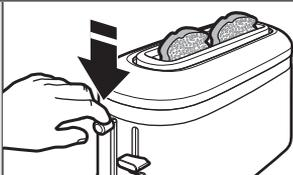
With the shade control lever set to your desired shade, press down on the high lift lever to start the toasting cycle.
