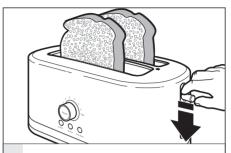
Press down on lift lever to lower the 2 toast back into the Toaster.
