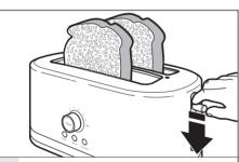
Press down on lift lever to start the toasting cycle. If Keep Warm isn't selected, the toast will rise automatically at the end of the cycle and the Toaster will turn off.
