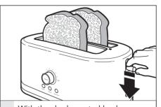
With the shade control knob set to your desired shade, press down on the lift lever to start the toasting cycle.
