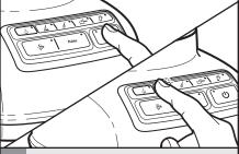
Press and hold a speed button for the desired length of time. Both the speed button and PULSE (Pulse) mode indicators will stay lit when pulsing. Blending will stop when Pulse button is released and the Pulse indicator will resume blinking. To pulse again at another speed, just press and hold the desired speed button.
